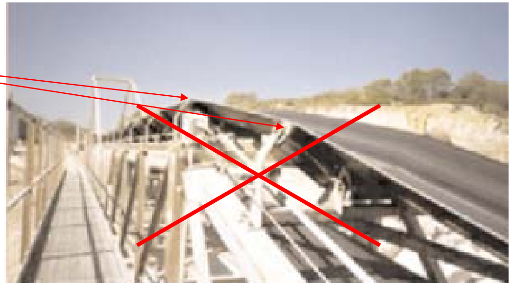
Figure 10. Typical guards at bend of conveyor
